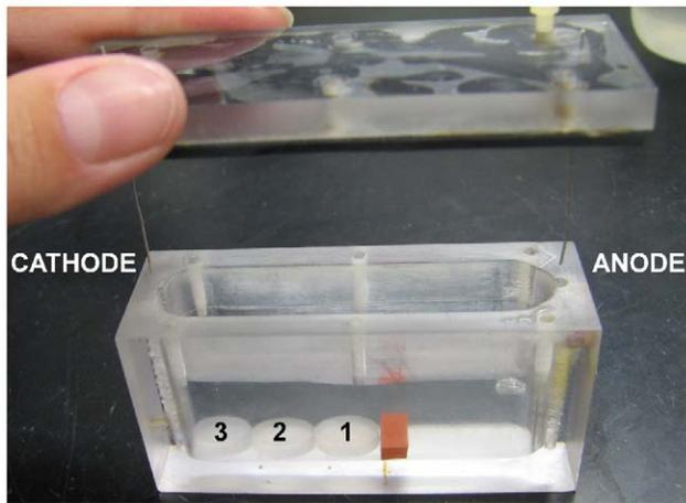
**Figure 1. Polycarbonate treatment well.** A piece of rubber sheeting on the bottom of the well held the biofilm-coated coupons at the same position (labeled 1–3) for each experiment. Platinum electrodes were inserted through the lid at opposite ends of the well and current was applied lengthwise. The anode was connected to the positive terminal of the power supply and the cathode to the negative. doi:10.1371/journal.pone.0055118.g001
