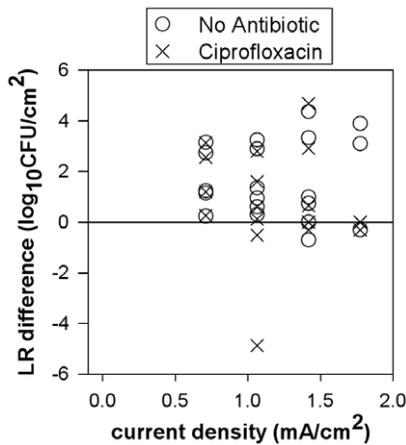
**Figure 3. Increased killing of *S. epidermidis* biofilm adjacent to the cathode.** Within each well, a trend of larger reductions at coupon 3 (adjacent to the cathode) compared to coupon 1 (near the center of the well) was observed following electric current treatment, as indicated by positive values. Each symbol denotes the measurement of the difference in LR between the extreme coupon positions (coupon 3 minus coupon 1) in a current-exposed well. doi:10.1371/journal.pone.0055118.g003
