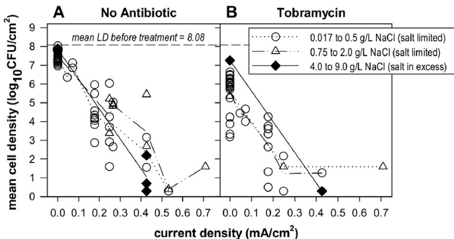
**Figure 7. Treatment of *P. aeruginosa* biofilm with direct current.** Direct current was applied to biofilm in wells containing (A) no antibiotic and (B) 10  $\mu\text{g}/\text{mL}$  tobramycin sulfate for 20 hours. All wells contained 0.1 g/L TSB with varying amounts of total NaCl. References to theoretical salt limitation or excess salt apply only to wells with current. Each symbol indicates a mean LD on coupons across one well and lines show connected means for each current level.
